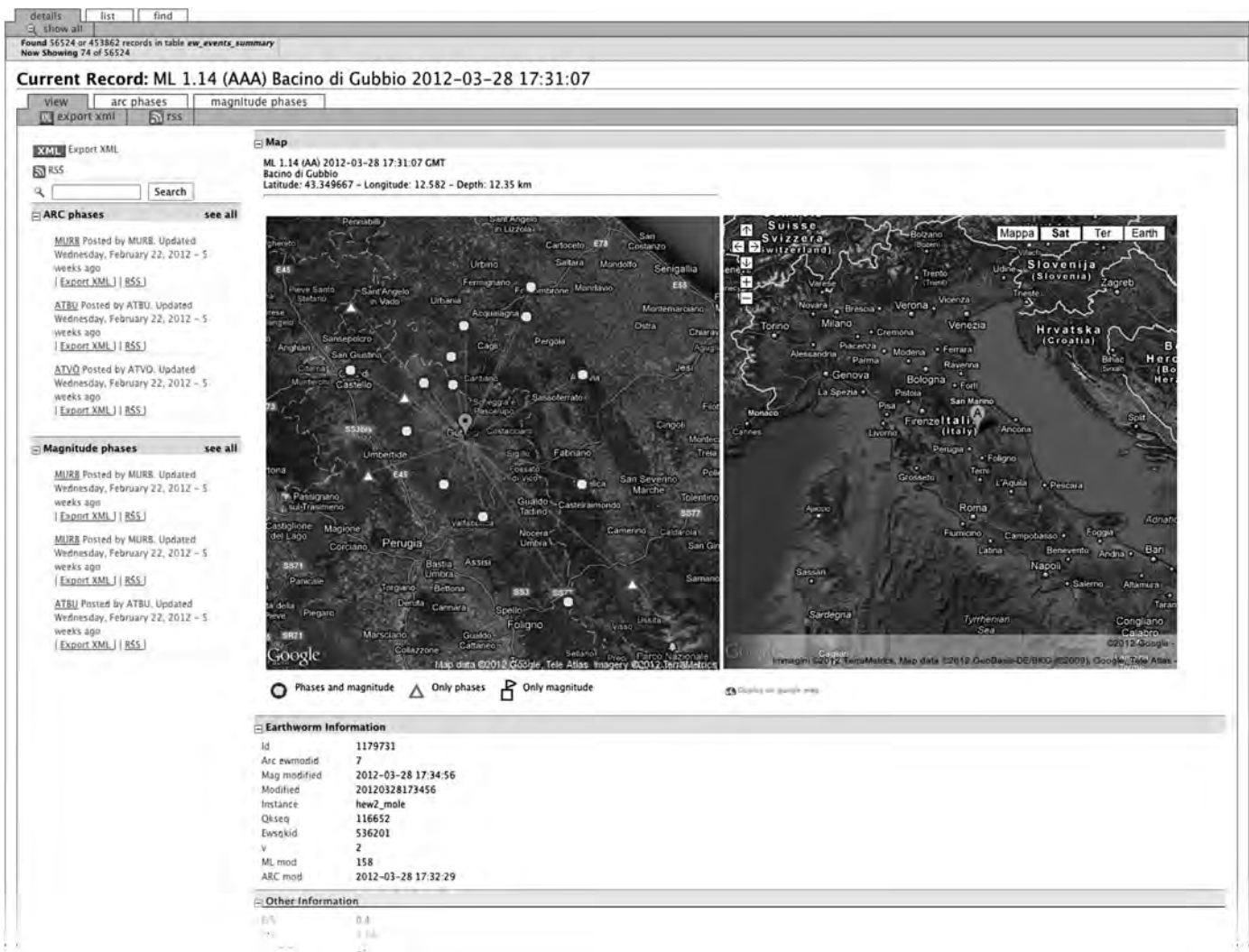
▲ Figure 5. Moleface earthquake location details. The page reports all available information about a single earthquake location and shows on the map the epicenter and the stations contributing only to location (triangle), only to magnitude estimate (square with flag), or both (circle). You can reach detailed information about the location and magnitude phases by clicking on the corresponding link.
