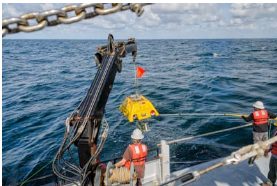
Researchers on the Research Vessel Oceanus retrieve an ocean-bottom seismometer during a 2014 expedition supporting the Cascadia Initiative.
